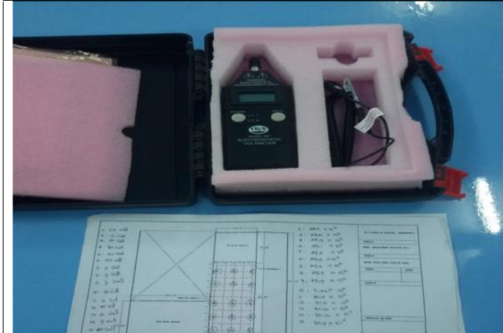
TAHAP-14 : TEST UJI GROUND RESISTANCE (Ohm) & FRICTION VOLTAGE (Volt)
