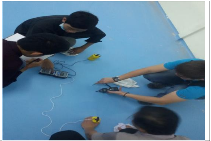
TAHAP-16 : TEST UJI GROUND RESISTANCE (Ohm) & FRICTION VOLTAGE (Volt)
