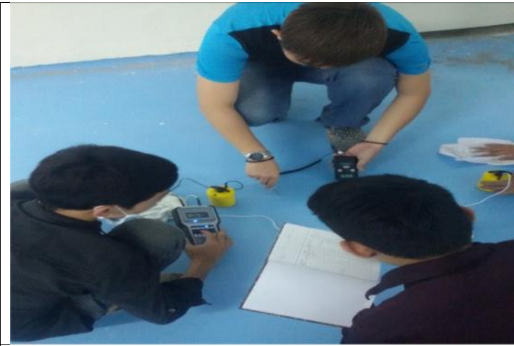
TAHAP-16 : TEST UJI GROUND RESISTANCE (Ohm) & FRICTION VOLTAGE (Volt)
