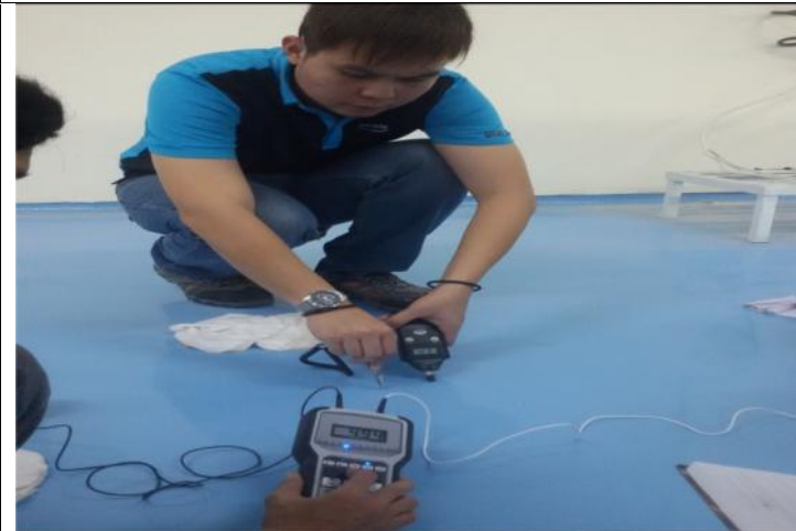
TAHAP-17 : TEST UJI GROUND RESISTANCE (Ohm) & FRICTION VOLTAGE (Volt)
